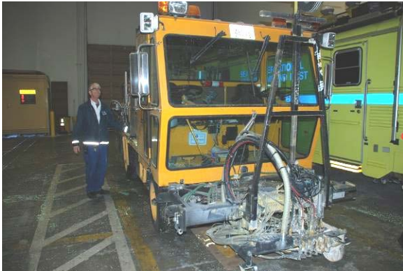
Purpose-built striping truck.
