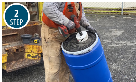
2 STEP Drill a hole in the barrel's lid. Make sure it is offset so it doesn't flow directly into the interior pipes.
